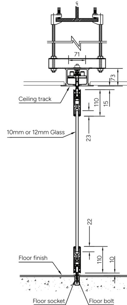
**Vertical Section of Panel & Track Fixing**
